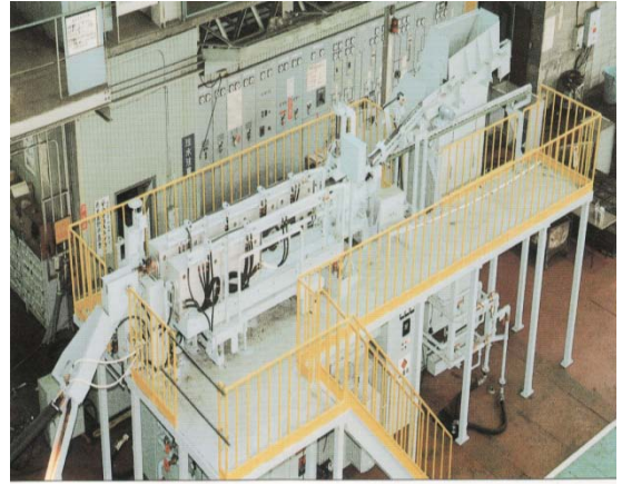
750KW 3000Hz modular type billet heater
